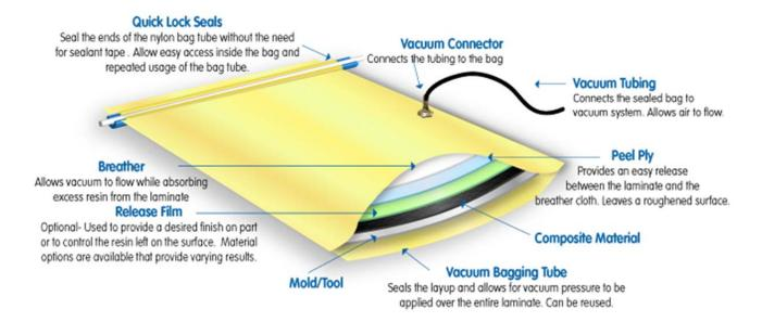
The Quick Lock Seals are a quick, convenient, innovative method of sealing the nylon bag tube without the need of a sealant tape. The tube can then be reused with no loss of material.
